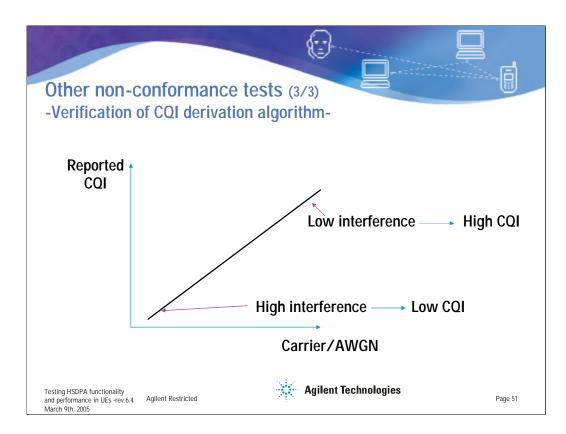
Once the derivation algorithm has been created, the designer can also verify the functionality of the CQI derivation algorithm by configuring the HS-DSCH according to a certain CQI value and checking that the reported CQI varies as expected for different AWGN levels.
