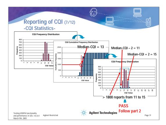
Once 2000 reported CQI values have been received from the UE and decoded, the frequency distribution of the reported CQI value must be analyzed. For stable conditions, the variance of the CQI report must be within certain limits. Out of 2000 CQI values, more than 1800 must fall within a range of 5 CQI consecutive values (from a value of (median CQI – 2) to a value of (median CQI + 2).
