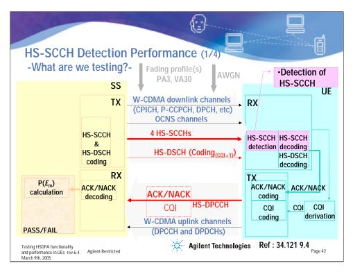
The purpose of the Detection of HS-SCCH test is to ensure that the UE is capable of correctly recognizing when it is being signaled by an HS-SCCH.
