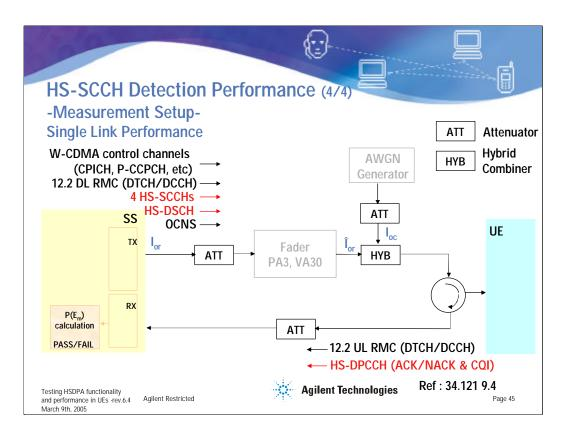
The generic connection diagram for the HS-SCCH detection performance conformance test is shown above. Fading profiles and AWGN might be provided by the system simulator itself, or if not available, by external faders and AWGN sources.
