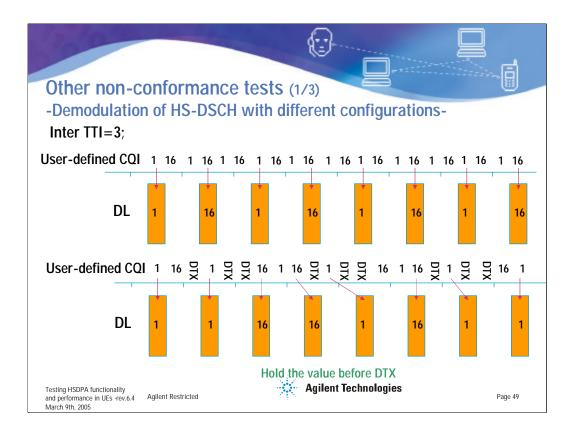
Even though the Demodulation of HS-DSCH conformance test requires a certain fixed channel (fixed modulation and coding), in early design verification different fixed configurations or a more dynamic channel configuration with the coding parameters changing according to the CQI report might be needed to test the UE decoding capabilities thoroughly.
