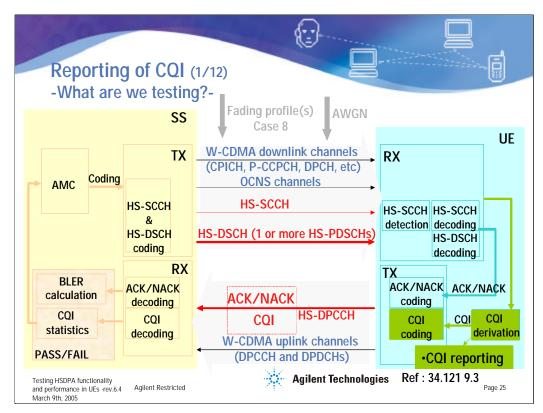
The Reporting of CQI tests evaluate the accuracy of the CQI reporting under different AWGN and fading conditions. The CQI reporting function mainly consists of the CQI derivation algorithm and the CQI coding.
