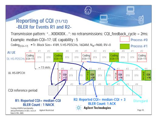
This slide shows an example of the procedure to calculate BLER for events R1 and R2.
