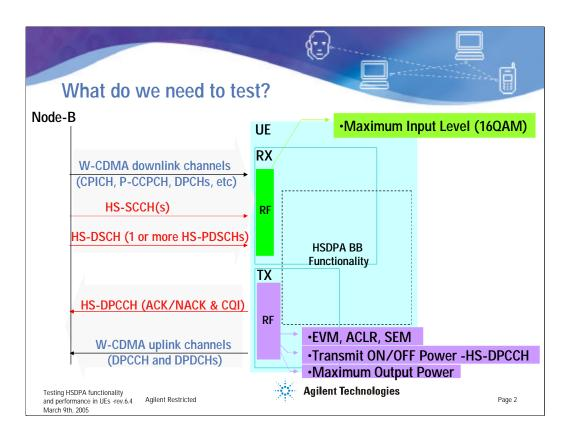
HSDPA is an addition to W-CDMA which mainly affects the downlink. The new downlink and uplink channels are highlighted in red in the slide. This has two implications:
