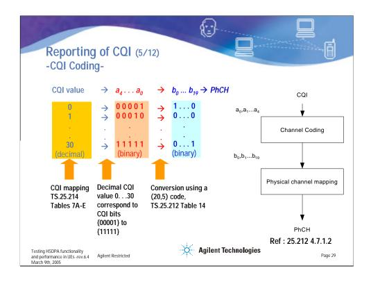
Until now, the CQI value derivation procedure in the UE and the relationship between a CQI value and the corresponding HS-DSCH coding configuration has been reviewed. This slide illustrates the CQI coding process in the UE.
