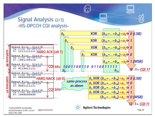
The demodulated bits for the CQI field can also be examined and the CQI field manually decoded, although this involves a lengthier and more cumbersome process, as shown earlier.
