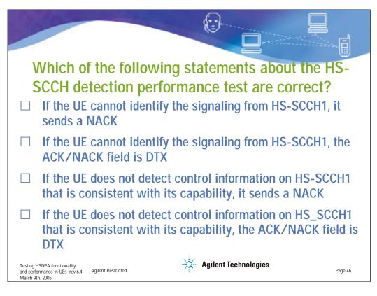
Which of the following statements about the HS-SCCH detection performance test are correct? □If the UE cannot identify the signaling from HS-SCCH1, it sends a NACK
