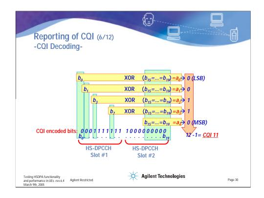
During the first part of the Reporting of CQI under AWGN propagation conditions test, the HS-DSCH TF (corresponding to CQI=16) is fixed and 2000 blocks are sent to the UE. The CQI values reported back from the UE must be decoded and collected in order to calculate the reported CQI value statistics. The CQI decoding takes place in the SS as part of the conformance test procedure in the specifications.
