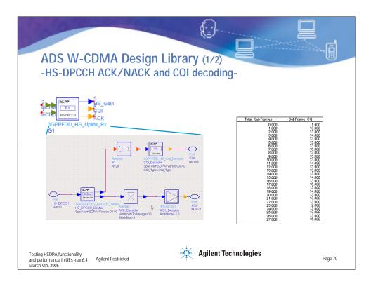
If ADS is available, connectivity between ADS and the Agilent signal analyzers and logic analyzers can be used to obtain a longer capture of the uplink signal and transfer it to ADS, as mentioned earlier. The behavioral HSDPA decoder in the ADS W-CDMA design library can perform the ACK/NACK and CQI decoding, without the need of a user-programmed method.
