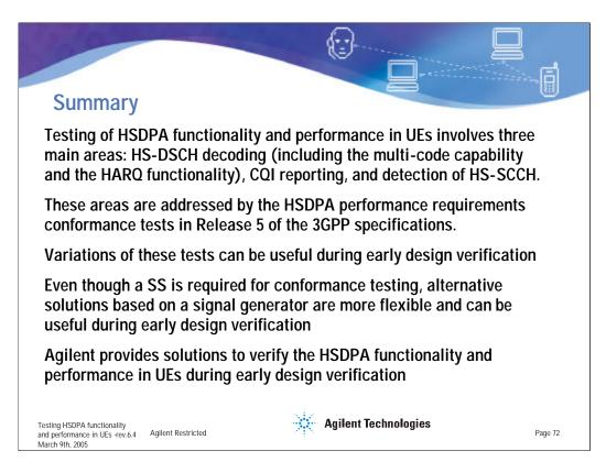
As a summary, testing of HSDPA functionality and performance in UEs involves three main areas of the UE functionality, which coincide with the more challenging aspects of the new HSDPA functions: the HS-DSCH decoding (including the multi-code demodulation capability and the HARQ functions, such as the IR combining, that take place during the decoding process), the CQI reporting (including the CQI derivation algorithm and coding), and the detection of the HS-SCCH.
