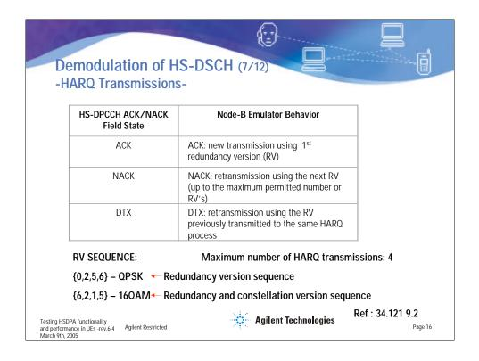
The slide shows the response of the SS to an ACK/NACK, as described in the Demodulation of HS-DSCH conformance test specifications. The objective is to simulate the behavior of the Node-B. Upon receiving an ACK, the SS must send a new block of data. Upon receiving a NACK, it must send a retransmission using the next RV (up to the maximum number of RVs allowed). Upon receiving a DTX, the SS will retransmit the same block of data using the same RV previously transmitted for the same HARQ process.
