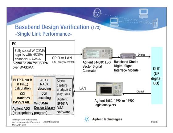
If the DUT has digital inputs or outputs, a similar measurement setup can be used to perform the HSDPA tests discussed. Agilent Studio for HSDPA over W-CDMA is used in combination with the Agilent E4438C ESG vector signal generator to generate W-CDMA downlink signals with fully coded HSDPA channels. The Baseband Studio Digital Signal Interface Module (DSIM) is used to provide fast digital inputs and outputs for the E4438C ESG vector signal generator.
