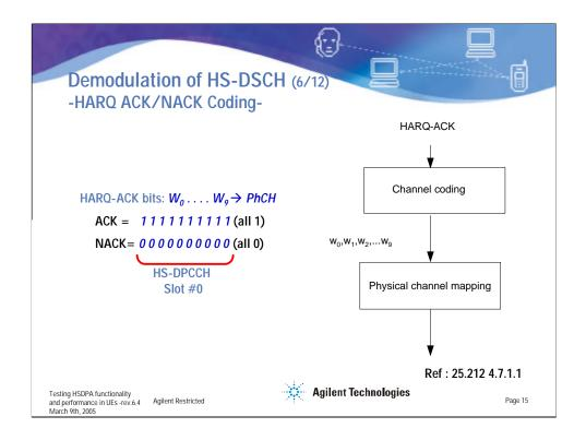
The UE indicates successful reception and decoding of a block by sending an ACK. If payload is received, but damaged and cannot be decoded, the UE reports a NACK. If the UE is not expecting data or decides that the data is not intended for it, it does not send either an ACK or a NACK.
