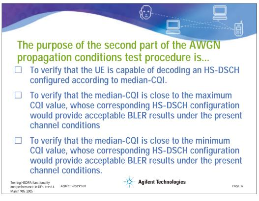
The purpose of the second part of the AWGN propagation conditions test procedure is...
