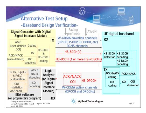
A similar setup can be used if the DUT has digital inputs/outputs. The main differences is that the signal generator must have digital outputs and that a logic analyzer (or some kind of digital signal interface) should be used instead of the signal analyzer to capture the uplink signal prior to decoding. If using EDA software, it is advisable to use a logic analyzer or digital signal interface module that has connectivity to the EDA software tool.
