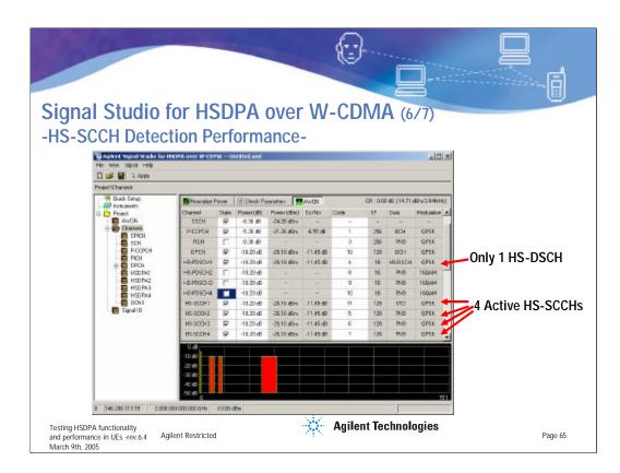
The most important feature for the HS-SCCH detection performance test is the ability to transmit HS-SCCHs without the presence of associated HS-DSCHs. Signal Studio for HSDPA over W-CDMA provides this capability, as shown in the slide. According to this measurement setup, 4 HS-SCCHs are transmitted, while only 1 HS-DSCH is transmitted, as required by the specifications for this test.
