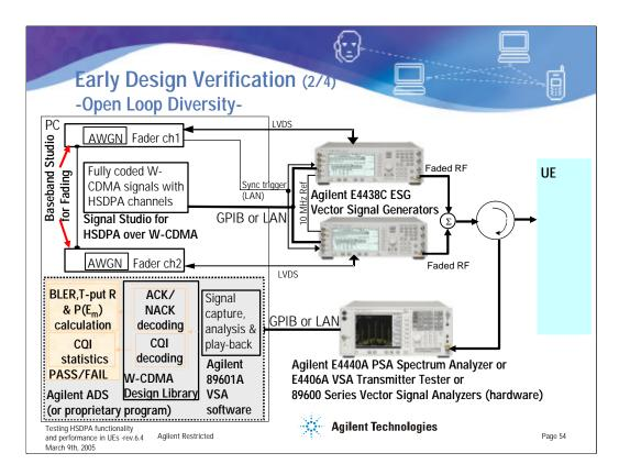
Alternative solutions for open loop diversity based on signal generators require two signal generators, one for each antenna. The two signal generators must be synchronized, so that the correlation between the antennas can be precisely controlled, which simulates the physical distance between the two antennas.
