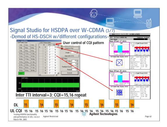
Signal Studio for HSDPA over W-CDMA allows the HS-DSCH to be configured according to different CQI values (so different modulation and coding) for every subframe. This feature can be used during early design verification to test the UE's capability to decode the HS-DSCH with different fixed configurations or with configurations that vary according to the user-defined CQI pattern in order to simulate a dynamic AMC environment.
