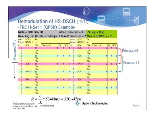
A theoretical example of the measurement results for the FRC H-Set 1 (QPSK) is shown above. As in the shorter example earlier, the maximum number of HARQ transmissions is 2 and the RV sequence is {0,2}.
