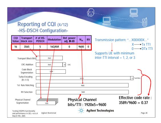
It the transport block size, the number of HS-PDSCHs, and the modulation scheme are known, the number of physical channel bits and the effective coding for the HS-DSCH can be determined, as shown earlier in the presentation. The same three parameters, along with  $N_{IR}$  and the RV parameter, define the whole HS-DSCH coding.
