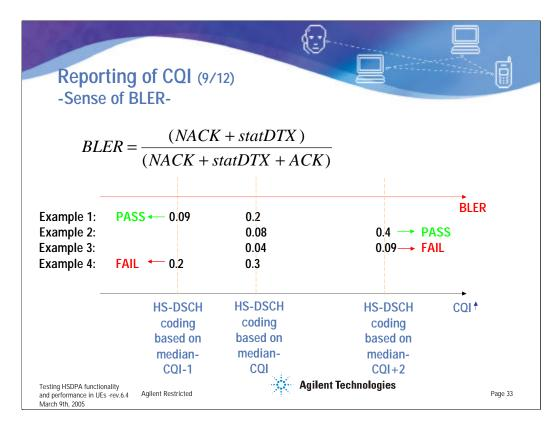
For the Reporting of CQI under AWGN propagation conditions test, as for the Demodulation of HS-DSCH test, BLER is defined as the ratio of unsuccessfully received and decoded blocks to the total number of information blocks sent. So, BLER is equal to (NACK + statDTX) / (NACK+ statDTX + ACK) as shown the slide.
