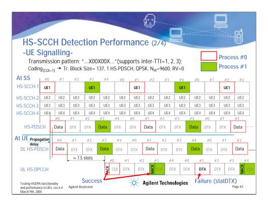
The slide shows as example of the procedure for testing HS-SCCH detection performance. The HS-SCCH1 TTI transmission pattern for this test is defined as "...X00X00X..." to accommodate UEs with minimum inter-TTI interval=3 (and lower). Two parallel processes must be used to support this pattern.
