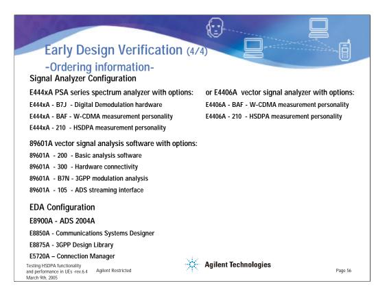
This slide provides the signal analyzer and EDA configuration for early design verification (single link performance and open loop diversity).
