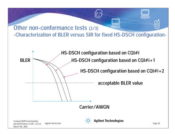
During the design of the CQI derivation algorithm, characterization of the BLER versus the Signalto-Interference Ratio (SIR) for each HS-DSCH configuration based on each CQI value might be required to determine the maximum CQI whose corresponding HS-DSCH configuration results in an acceptable BLER value for a certain SIR.
