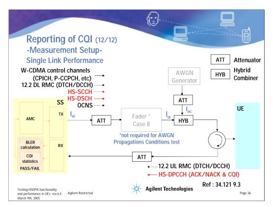
The generic connection diagram for the Reporting of CQI tests is shown above. Fading profiles and AWGN might be provided by the system simulator itself, or if not available, by external faders and AWGN sources. Note that fading is not required for the AWGN propagation conditions test. Both AWGN and fading are required for the Fading propagation conditions test.
