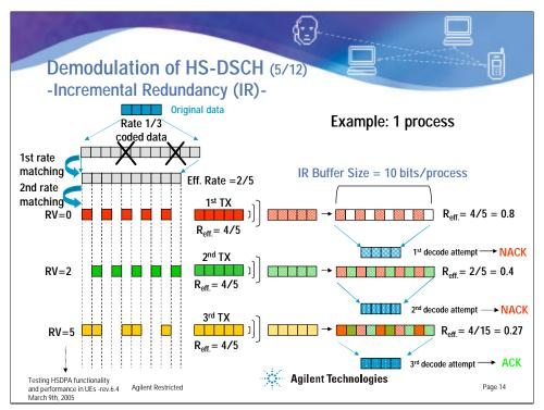
In order to understand the meaning and significance of the demodulation of HS-DSCH test it is useful to review some of the key elements of the HS-DSCH coding, in particular, the HARQ functionality and the IR combining scheme. This slide uses an example to demonstrate how the IR combining scheme works. For simplicity, an IR buffer size of 10 bits/process and a single process will be assumed.
