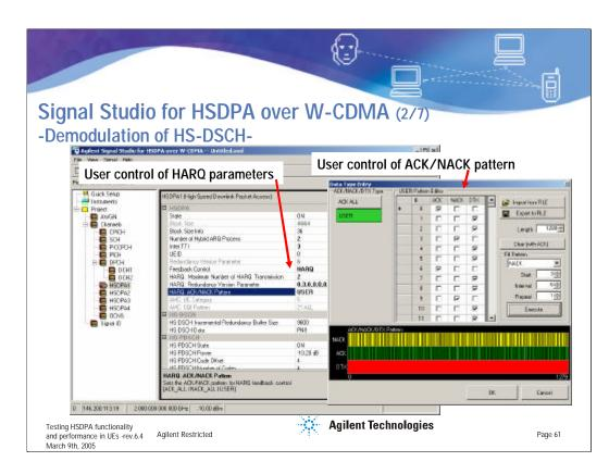
The Demodulation of HS-DSCH test requires the SS to react to the ACK/NACK report of the UE by transmitting new data or retransmitting the data block accordingly. As mentioned earlier, the signal generator cannot react to the true ACK/NACK report from the UE, because of the lack of a feedback loop. Therefore, the Demodulation of HS-DSCH test cannot be performed as required if a signal generator-based solution is used.
