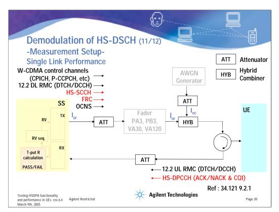
The generic connection diagram for the Demodulation of HS-DSCH, single link performance conformance test is shown above. Fading profiles and AWGN might be provided by the system simulator itself, or if not available, by external faders and AWGN sources.
