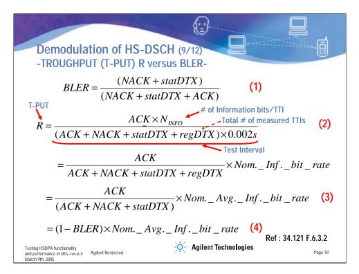
Block Error Ratio (BLER) is the metric used for most W-CDMA performance requirement tests. BLER is defined as the ratio of unsuccessfully received and decoded blocks to the total number of information blocks sent. In the case of HSDPA, BLER is equal to (NACK + statDTX) / (NACK+ statDTX +ACK) as shown in equation (1).
