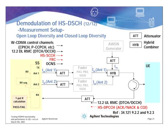
The HS-DSCH demodulation/decoding performance of the UE must also be evaluated under open loop and closed loop diversity scenarios. Diversity modes are part of the W-CDMA system, so they are not HSDPA additions. But the HSDPA performance will vary from single link scenarios, so different test settings and minimum requirements are given for diversity conditions.
