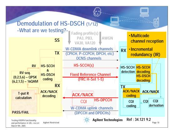
The Demodulation of HS-DSCH test is equivalent to the demodulation performance requirement tests for W-CDMA dedicated channels. It tests the HS-DSCH decoding performance of the UE, in particular the most challenging aspects: multicode channel reception and the IR HARQ combining scheme.
