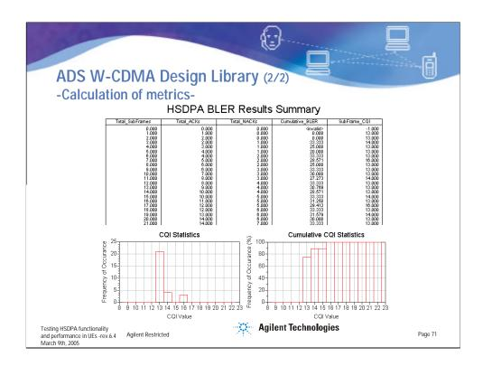
ADS also allows further processing of the decoded ACK/NACK and CQI values. Equations and graphics can be created to calculate the different metrics. The BLER calculation for an uplink signal example generated with Signal Studio for HSDPA over W-CDMA is shown in the slide. The CQI frequency distribution and cumulative frequency distribution that are needed to calculate the median and variance of the CQI are also shown.
