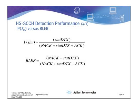
The probability of event  $E_{m'} P(E_m)$ , is defined as the ratio between the number of failures and the total number of blocks measured. So,  $P(E_m)$  is equal to statDTX/(NACK+statDTX+ACK).
